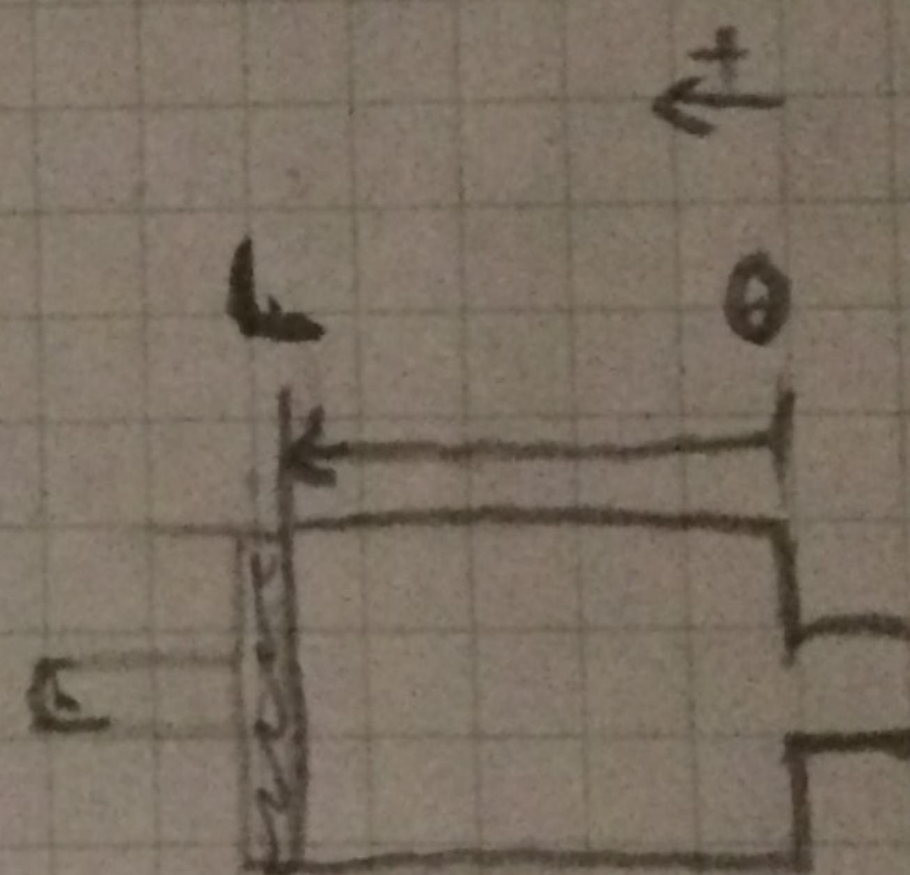
$$-\frac{\partial L}{\partial t} = \frac{0.9 Q_2}{A_p} = \frac{0.9 (300 \times 10^3 \text{ mm}^3 / \text{dk})}{500 \text{ mm}^2}$$
